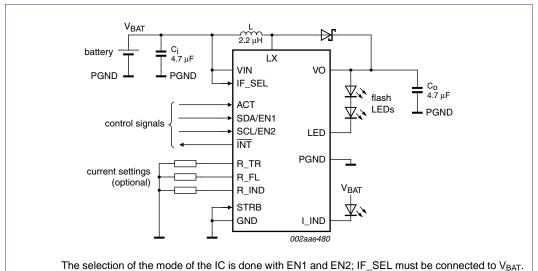
Fig 4. Typical application diagram of SSL3250A using Direct control only
