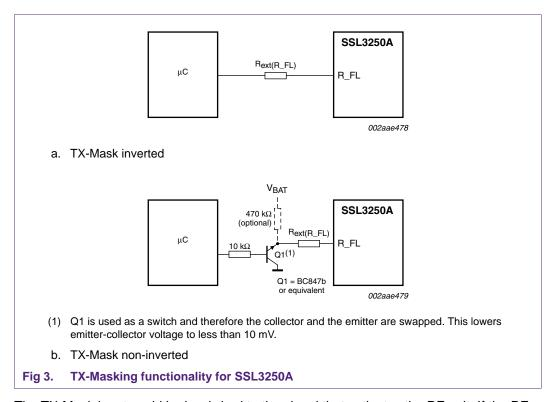
The TX-Mask input could be hardwired to the signal that activates the RF unit. If the RF unit is activated, the SSL3250A should reduce its power usage to make sure the battery is not overloaded. The timing of the SSL3250A has been matched to the general behavior of RF units.
