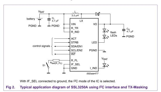
Using the SSL3250A as shown in Figure 2 provides a possibility to reduce the maximum output current of the LED driver in I<sup>2</sup>C mode, without changing the digital value stored in the current control register. This option could be useful in the situation to prevent the driver from using maximum power when the transmitter is being used. An external resistor can be connected to R\_FL to lower the output current to a defined level, which limits the total battery load to an acceptable level.
